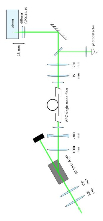
Figure 5.2 Speckle beam optics. The photodetector is used to monitor and stabilize the beam power (via feedback to the AOM RF power). Distances are not to scale.
