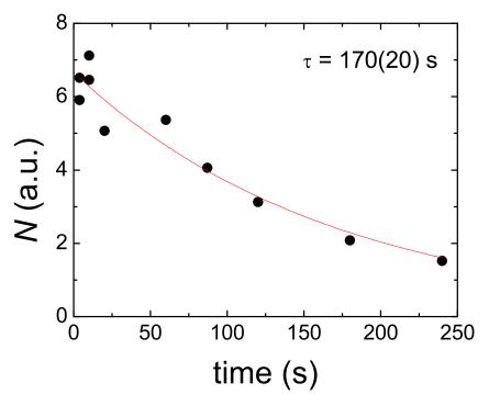
**Figure 2.13** Lifetime of trapped atoms in the science cell. The red trace is an exponential fit, which yields a 1/e decay time  $\tau$  of nearly three minutes. The temperature of the atoms is several hundred  $\mu$ K, high enough to make Majorana losses from the quadrupole trap negligible.
