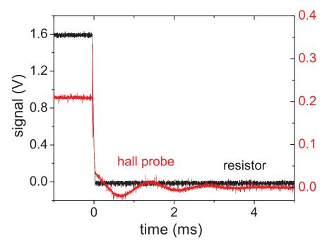
**Figure 2.10** Ringing of closed-loop Hall probe current sensor in response to a sudden change in current. No ringing is detectable in the voltage drop across a sense resistor.
