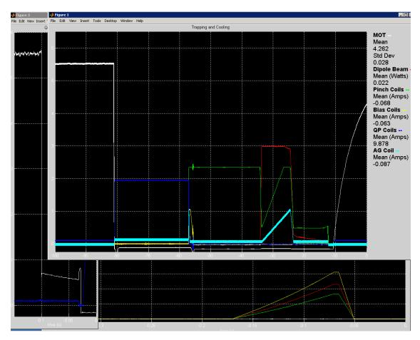
Figure 3.5 Screenshot of experiment monitor software. In the layout shown here, the main window displays the previous 100 seconds of operation, including one cycle of an experiment loading a BEC into a 3D optical lattice. The lower window shows the lattice beam intensity for +50 ms, -300 ms (partially obscured) around the release of the atoms. The left window shows the MOT to quadrupole trap transfer (section 2.8).
