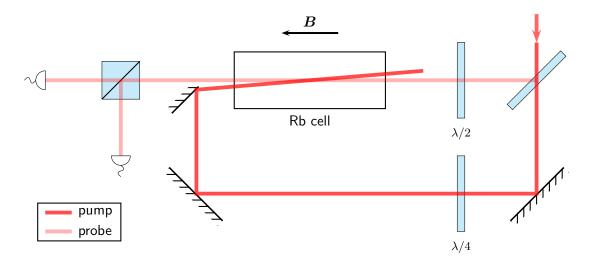
**Figure 2.5** Polarization spectroscopy setup for laser stabilization. The pump beam is circularly polarized while the probe beam is linearly polarized.
