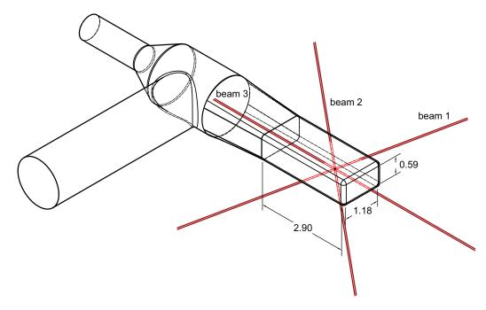
**Figure 2.8** Isometric view from above of science cell; dimensions are in inches. The rectangular cross-section enables very high numerical aperture optical access from the top and bottom. This figure also shows the paths of the optical lattice beams (chapter 4).
