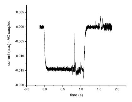
**Figure 2.16** Sudden jumps in current through the Ioffe bars during and after a slow ramp down of the setpoint current. Note that the signal here is AC-coupled, so the ramp appears as a constant offset from zero between 0 s and 1.1 s.
