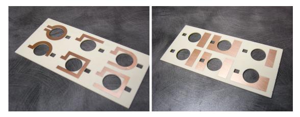
**Figure 6.10** Microwave coils as fabricated. The board was subsequently diced and each coil tested separately.
