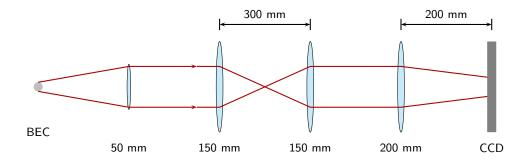
**Figure 2.24** Auxiliary imaging system. The path contains several mirrors, not shown, to wind it toward the camera. For simplicity, the unscattered absorption imaging probe beam light is omitted from the figure.
