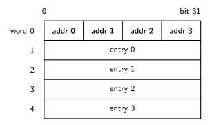
Figure 3.7 Data format generated by out\_fpga and used by plb\_fastdio core.
