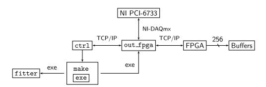
Figure 3.8 Schematic of control system software and FPGA sequencer. NI-DAQmx is the software driver for the PC-based analog output hardware (NI PCI-6733). For the description in section 3.1.3, out\_fpga is replaced by out\_pc, which communicates directly with driver for the PC-based digital output hardware (UEI PDL-DIO-64TS).
