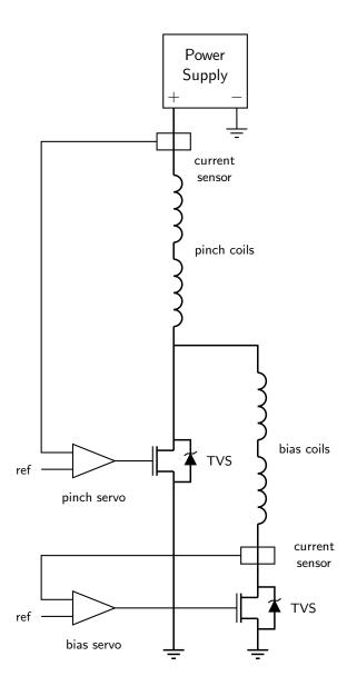
Figure 2.17 Schematic of IP trap circuit.
