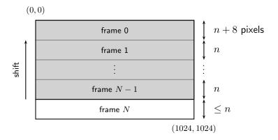
**Figure 2.23** Layout of CCD in kinetics mode for a Princeton Instruments VersArray XP camera. The shaded region is shielded from light using, e.g., a razor blade, and is used to store images taken by exposing the unshaded region. The value n can be set using the camera's software driver.
