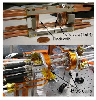
**Figure 2.14** Core portion of Ioffe-Pritchard magnetic trap (top). Current flows in opposite directions in neighboring sets of bars. Assembled trap showing bias coils and connections for current and cooling water (bottom).
