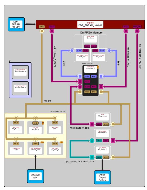
Figure 3.6 Structure of FPGA-based digital sequencer.
