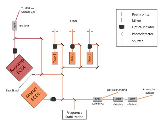
Figure 2.2 Schematic of diode laser system.
