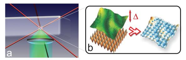
**Figure 5.1** Schematic view of (a) science cell showing speckle beam and optics and optical lattice beams (red) and (b) creation of disordered lattice by combining speckle field and clean lattice.
