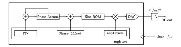
Figure 3.3 Schematic of a direct digital synthesizer. The FTW register determines the output frequency according to  $f = f_{\text{ref}} \times \text{FTW}/2^N$ , where N is the width of the FTW register. To keep the size of the sine ROM to manageable level, typically only the most significant 15–19 bits of the phase value are used.
