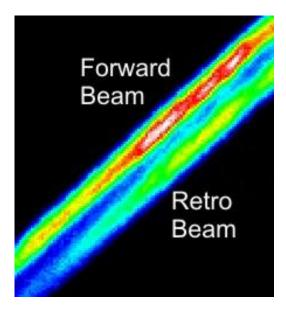
**Figure 4.7** Fluorescence from one lattice beam on resonance passing through hot atom cloud. The retro beam is not yet aligned.
