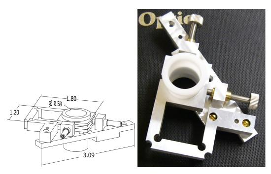
**Figure 5.5** CAD design of flexure mount for speckle lens and diffuser and image of finished mount. Representative dimensions (in inches) given to suggest scale.
