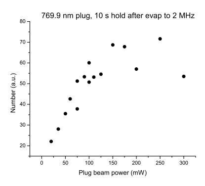
**Figure 2.28** Lifetime of cold atoms (after RF evaporation) in the plugged quadrupole trap vs. plug beam power. The beam is detuned by only -10 nm from the D2 resonance.
