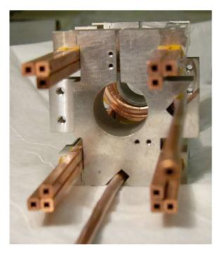
Figure 2.15 End-on view of Ioffe bars during construction.
