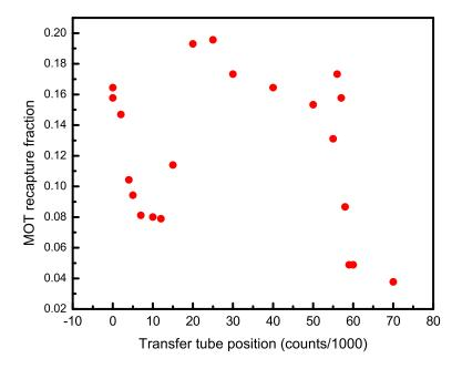
**Figure 2.12** Fraction of atoms recaptured in MOT after transport to given position in transfer tube and return. The initial dip is due to stray light, which is blocked once the atoms are inside the transfer tube. The loss around 58000 counts, just at the entrance to the welded bellows connecting the transfer tube to the science cell, is believed to result from stray magnetic fields.
