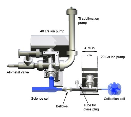
**Figure 2.7** CAD design for ultra-high-vacuum system. The ion pumps are Varian StarCell pumps. The glass cells (blue) were custom made by Technical Glass.
