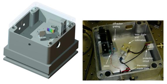
**Figure 2.3** CAD model and photograph of external cavity diode laser design. A thermoelectric element between the enclosure and the plate to which the ECDL components are mounted is used to adjust the temperature of the plate.
