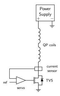
Figure 2.9 Schematic of quadrupole coil circuit.
