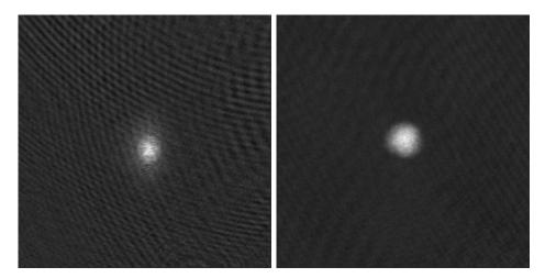
Figure 2.22 Sample images taken without (left) and with the quarter-wave plate installed in the imaging system.
