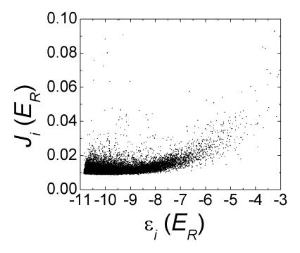
**Figure 5.11** Correlation between site energy  $\varepsilon_i$  and tunneling matrix elements averaged over all nearest neighbors,  $J_i$ .
