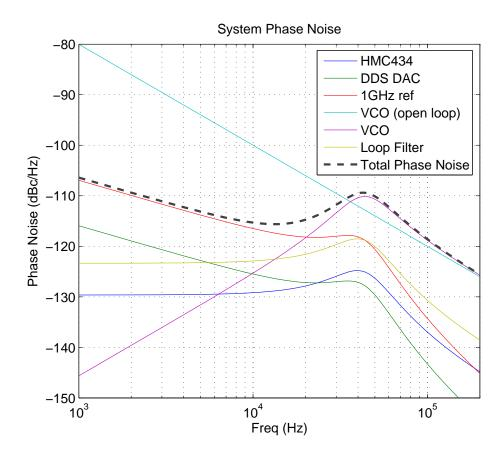
**Figure 6.9** Phase noise calculated for PLL shown in figure 6.8. The contributions for each component are shown for closed loop operation (VCO refers to the YIG oscillator, HMC434 to the frequency divider). The open loop VCO phase noise is shown for comparison. The loop design bandwidth (3 dB) is 50 kHz, with a phase margin of 40°.
