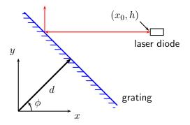
**Figure 2.4** Schematic of improved ECDL design. The grating is parameterized by  $y \sin \phi + x \cos \phi = d$  and the external cavity length is  $l = x_0 - (d - h \sin \phi)/\cos \phi$ . The wavelength selected by the grating angle is  $\lambda = 2a \sin \phi$ , where a is the grating period, while the wavelength selected by the cavity length is  $\lambda = 2l/m$ , where m is the number of waves in the cavity.
