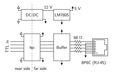
**Figure 3.4** Isolation circuit for digital signals. The DC-DC converter is a Texas Instruments DCP010512, the isolator is an Analog Devices ADuM1400, and the buffer is a generic 74ACT573.
