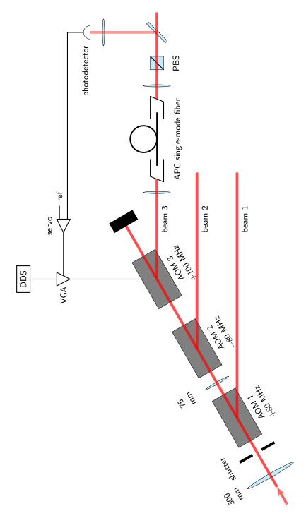
**Figure 4.5** Distribution of light for the optical lattice. Light from the Ti:Sa laser is picked off and frequency shifted by three AOMs. The intensity exiting the fiber is monitored by a photodetector and stabilized by feeding back to the RF power driving the AOM, as shown for beam 3. Identical systems (not shown) are used for beams 1 and 2. The DDS can be used to control the RF amplitude during open loop operation, e.g., for fast pulses.
