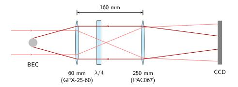
Figure 2.21 Optical system used for absorption imaging of atoms in science cell. The first lens is a Lightpath Gradium GPX-25-60, the second is a Newport PAC067 achromatic doublet. The predicted magnification is 4.06, with a spot diameter of 3.7  $\mu$ m. The quarter-wave plate (denoted  $\lambda/4$ ) prevents etaloning between optics on either side of it.
