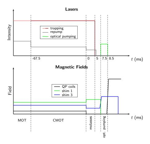
**Figure 2.11** Sequence for transfering atoms into quadrupole trap from the MOT. The axes are not to scale. Note that the trapping lasers are detuned further at the start of the CMOT stage (indicated by the change in trace color).
