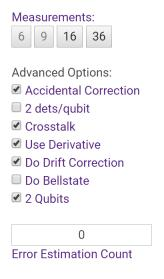
Step 2: Select the type of configuration needed for analysis of the dataset. In this example, a 1 detector per qubit, 16-measurement analysis with accidental correction, drift correction, and crosstalk will be performed. A 9-measurement tomography is only possible with 2 detectors per qubit. It is also advisable to always select 'Use Derivative when performing the calculation to speed up the calculation.
