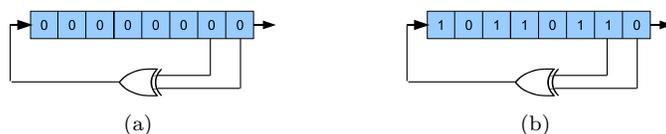
Figure 2.1: Examples of LFSR implementations with a seed state size of  $n = 2$  bits. Bits in (a) have been generated using a seed state of “00,” resulting in completely periodic results while bits in (b) have been generated using a seed state of “01,” resulting in the maximum period of  $2^n - 1$ .
