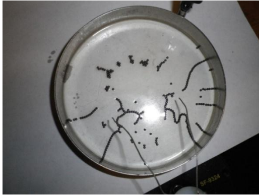
Fig. 2 11kV perimeter electrode & steel balls in castor oil
