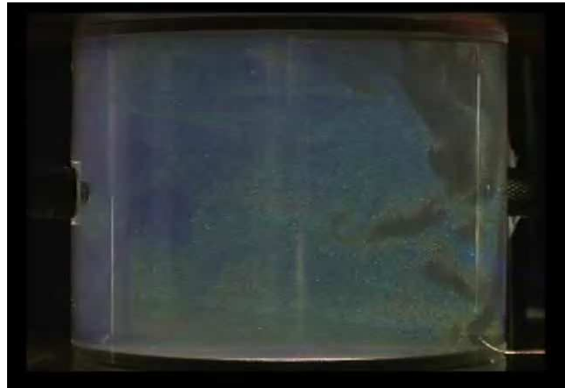
Experiment with water, Ra=3.7 \cdot 10^8 : Du and Tong, JFM (2000)
